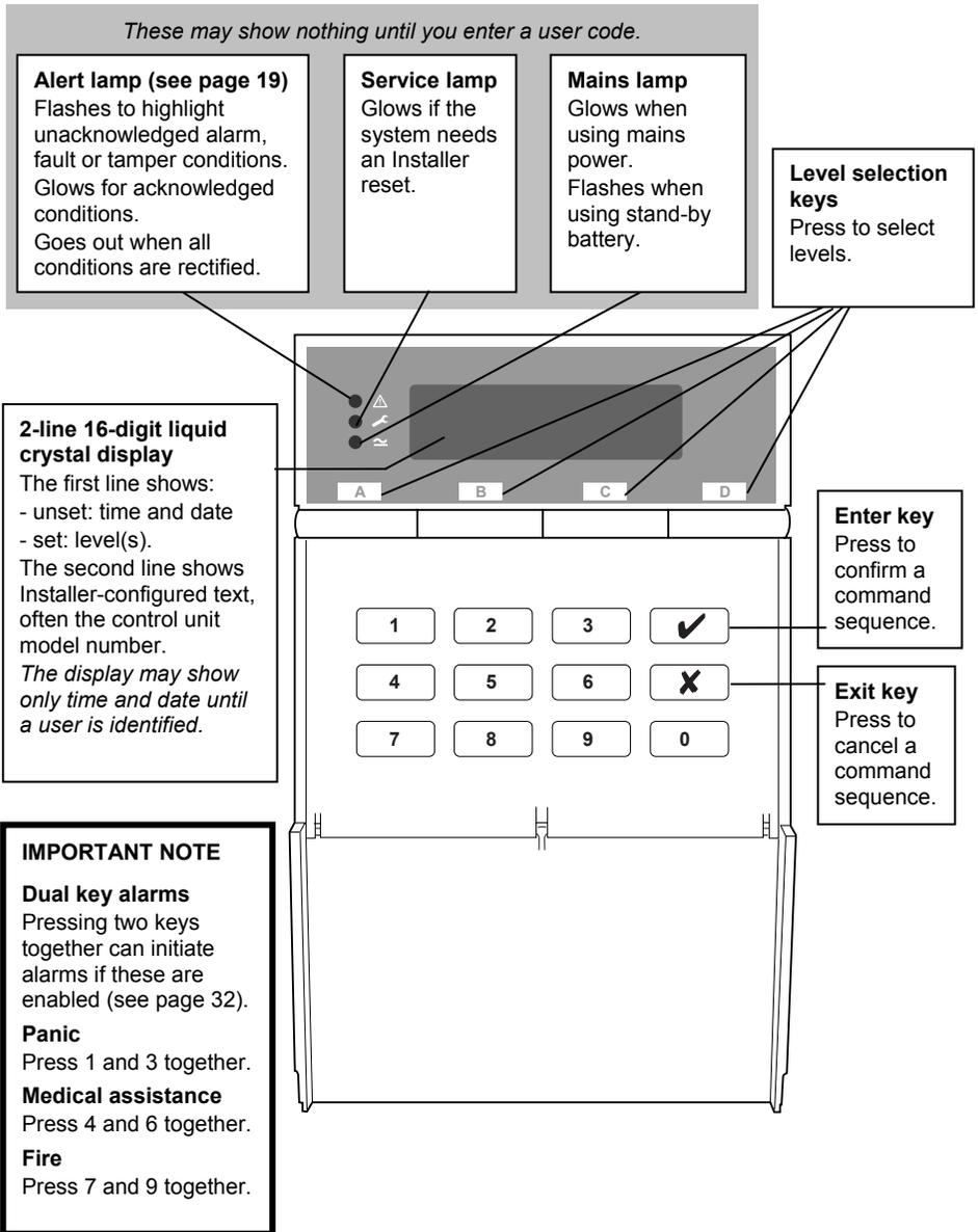
Figure 1. 9941 and 9943 LCD Remote Keypads
